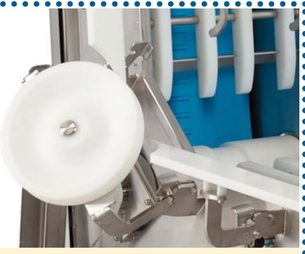
Fold out, rounded UHMW wheels to assist belt tracking.
