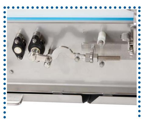
Easy to operate, belt tensioner to loosen belt prior to removing sideboards and activating belt lifting system
