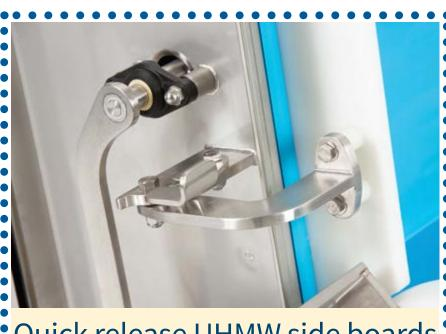
Quick release UHMW side boards mounted on hinges, captivated to conveyor frame. Eliminate potential for lost/ misplaced guides during sanitation process.
