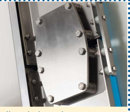
All wash-down duty components mounted on stand offs to meet sanitation requirements
